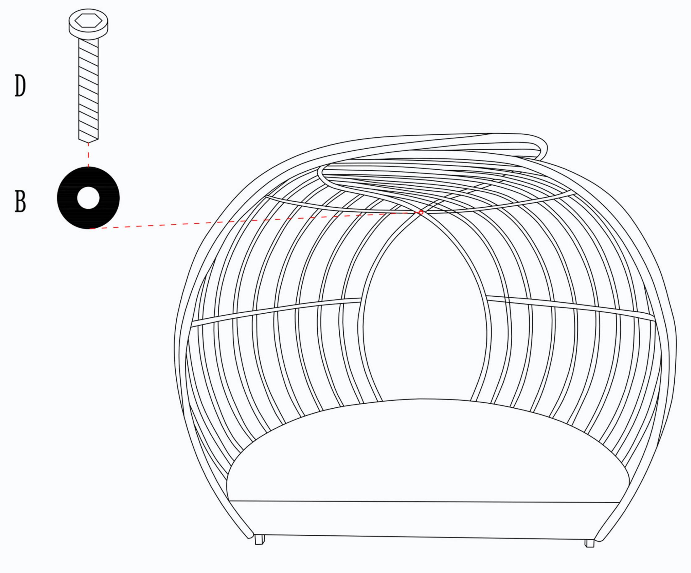
2 Screwing up all the screws tightening
